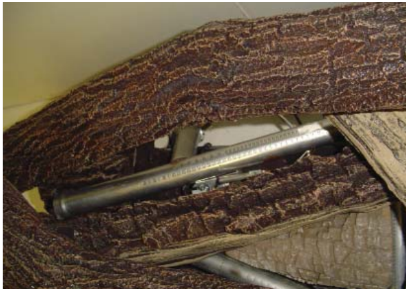
Figure 23A - Installing Back Top Log, Top View
