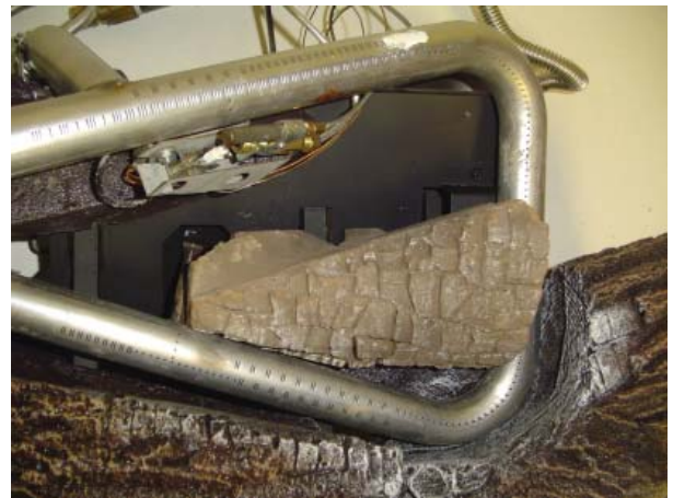
Figure 19A - Installing Charred Log Top View
